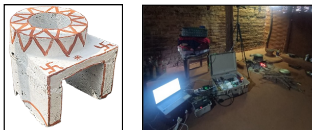
Fig. 1 PAVAK improved concrete cookstove and the sampling setup for source emissions monitoring
